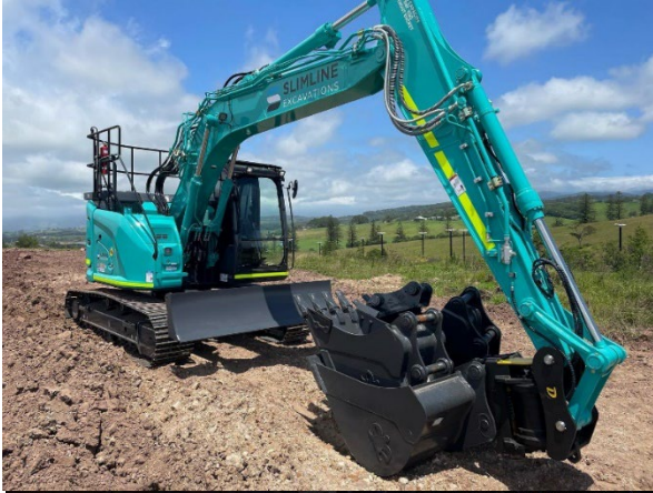
Slimline Excavations 14 tonne Kobelco Excavator bought in December 2021 with Doherty D-Lock Tilt hitch
