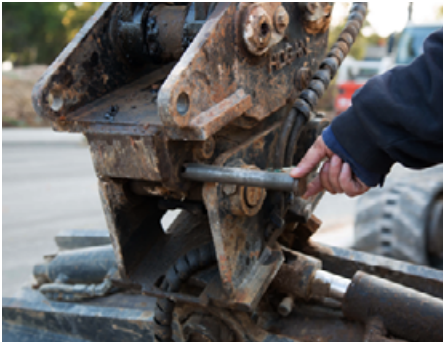
Photo 2: Shows a worker locating the safety pin for the semi-automatic quick hitch. This is an administrative measure, as it depends entirely on the action of the worker.
