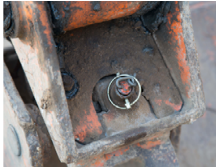
Photo 3: Another type of safety pin, in place and secured by a lynch pin to prevent it coming loose.
